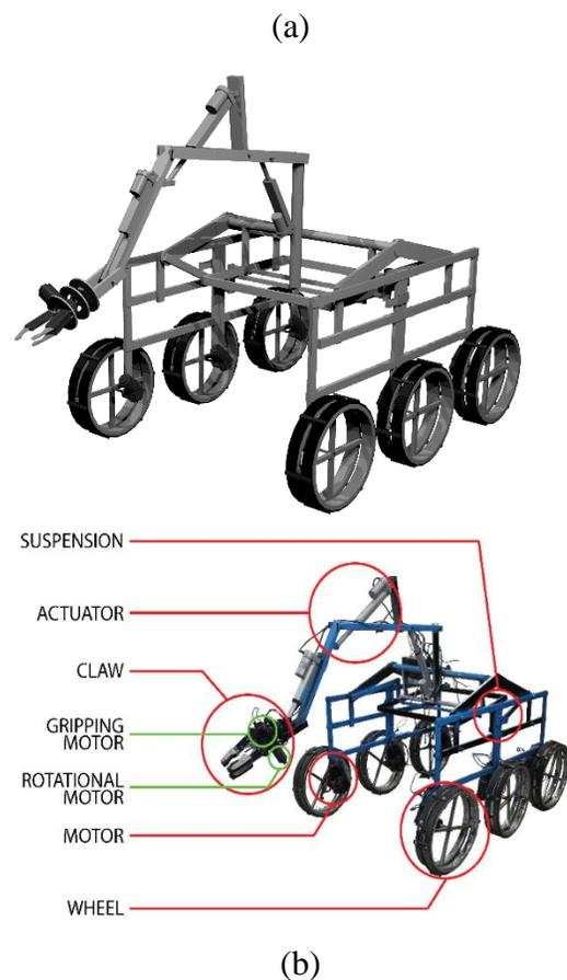
Fig. 1 (a) 3D design (b) Implemented model
